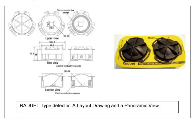
This detector type is dedicated to combination detection of radon and thoron activity at the same time.
